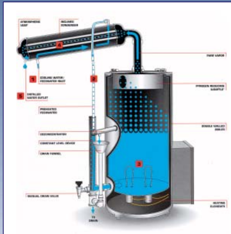
Typical electrically heated stills. Steam heated models also available.
