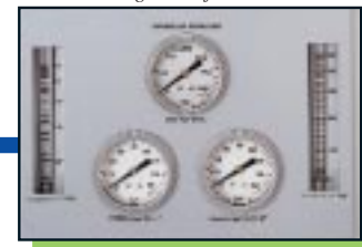
Pressure Gauges and flow meters
