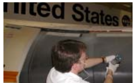
DG-2A being used to analyze the space shuttle's leading edge.
