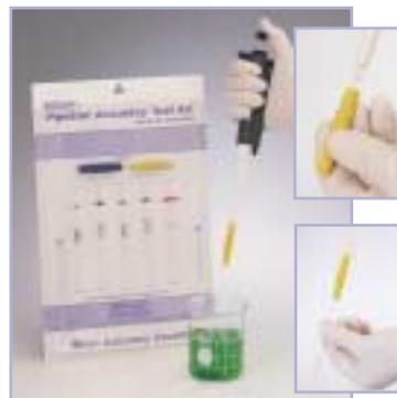
Pipettors trusted to deliver precise microliter volumes should be checked for accuracy on a regular basis. This test kit eliminates the time consuming alternative of using a balance. The kit is not meant for certification of calibration. It is ideal for all air displacement pipettors such as Rainin,
