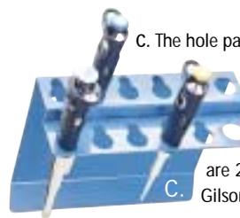
C. The hole pattern on this rack is the same as the Scienceware® H18962-0001 (B), but this rack is for wall mounting only. The back plate has two holes for screw attachment to the wall and double faced tape (included) on its lower edge. Dimensions are 229 x 98 x 203 mm H (9 x 3 3/4 x 8" H). Designed for Gilson Pipetman®. Plus the Drummond Pipette-Aid®.
