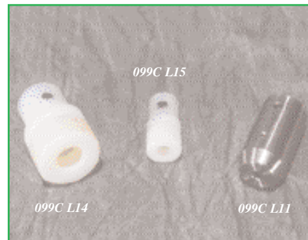
L14 and L15 fit Glas-Col motors or any motor with a 5/16" shaft. L11 chuck requires c.c.w. motor rotation.
