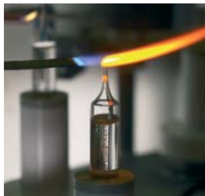
Our buffer solutions are hermetically sealed in double-pointed ampules and sterilized with superheated steam. You can rest assured that you will always have a reliable buffer solution on hand for calibration.
