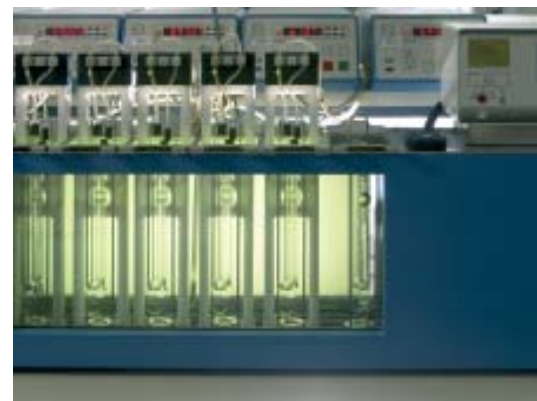
Each viscometer is calibrated and given an ID number and a certificate with its specific characteristics.
