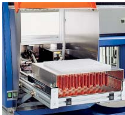
The electric sample lift ensures positioning of the samples in the rack at a convenient and easily monitored working height.
