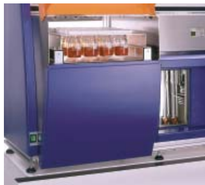
b) one rack with 16 positions to accommodate 100 ml sample bottles for normal volume applications
