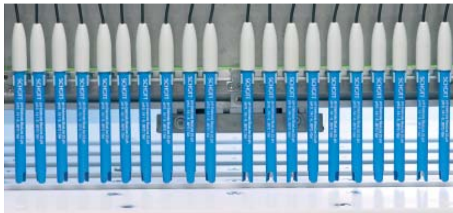
Thorough quality control checking is an essential element from start to finish. The zero point and response time of every electrode is checked – as shown here with a batch of BlueLine laboratory electrodes.
