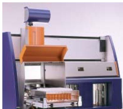
Two different sample racks are supplied: a) one rack with 56 positions for 20 ml sample bottles for micro-viscometer applications
